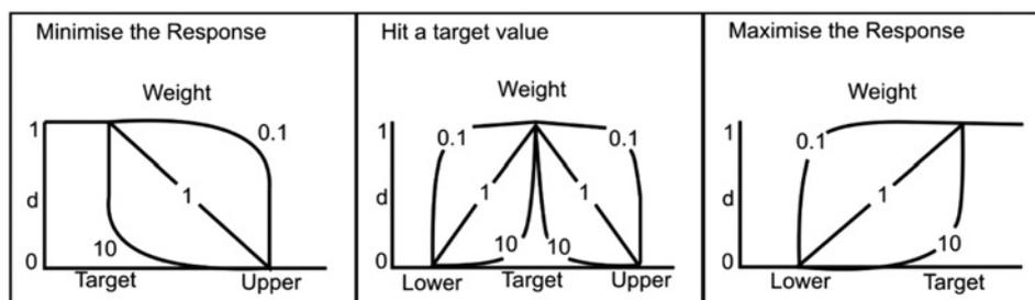
Fig. 3 Desirability functions for different goals—how Weights affect their shapes
